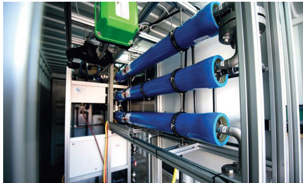
↑ The brine concentrator pilot with a multi-stage nanofiltration system up to 80 bars.
