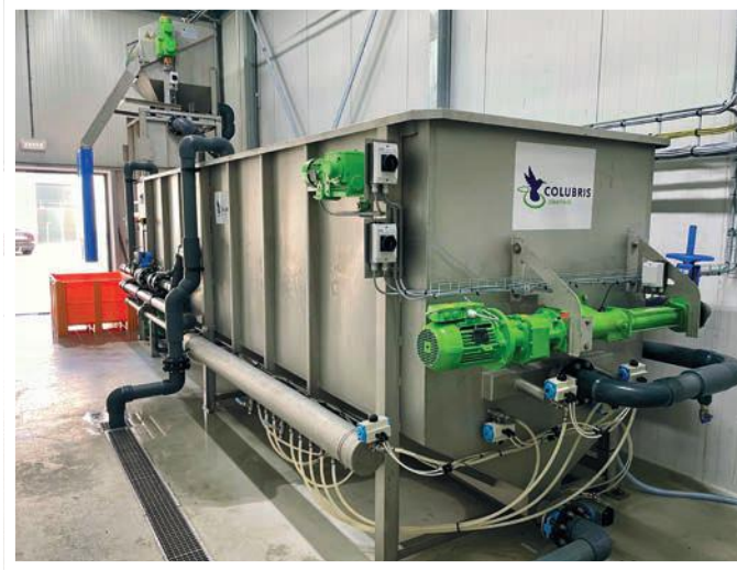
↑ → The water treatment of the Plukon site in Nijkerk (the Netherlands), consisting of a drum filter, polymer preparation unit and a DAF unit (Dissolved Air Flotation).
